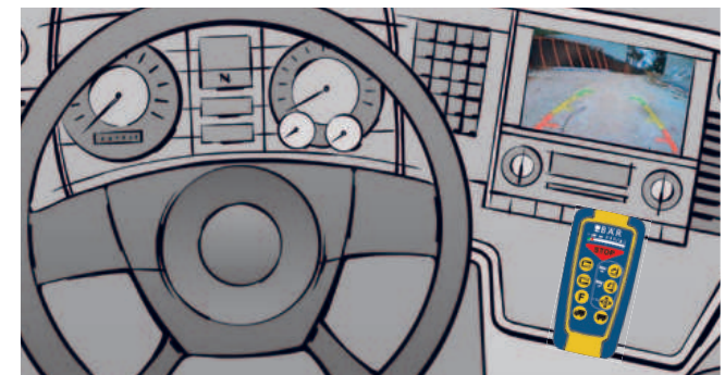
Bär SmartControl cabin control (option) for control of the Cargolift from the cabin by Bär SmartControl Plus with docking station. See technologies.
