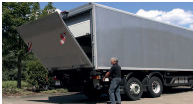
Bär rolling gate control (option) unit automatically opens and closes the rolling gate of the body depending on the Cargolift operation so that the cold air is kept inside the body and operation is made easier.
