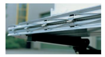
User-friendly manual folding of platform package and platform tip with spring relief (standard).
