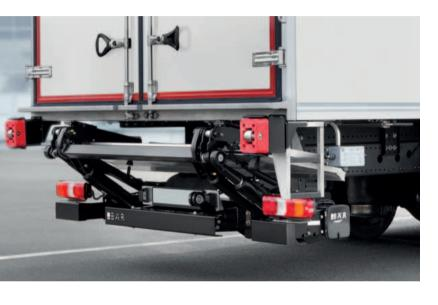
With manual unfolding with compact platform dimensions, the BC 1500 F offers a load capacity of 1500 kg and aluminium platforms with height of up to 1510 mm. Unlike F2 variants, it offers tilting compensation at every height by means of two tilting cylinders. In addition to user convenience, also safety is increased.
