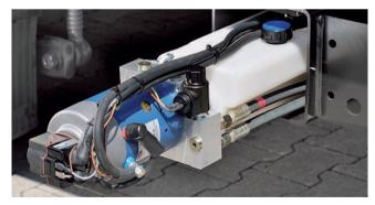
**Power pack and control unit** are safely protected in the beam (standard). Motor with thermal circuit breaker protecting against overheating and fire. Simple emergency operation of the four basic functions by pushbutton. **Low-noise power pack** (option) available.
