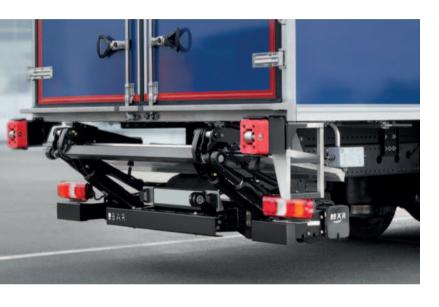
The manually unfolding BC 1000 F is a favourite solution for trolley transport with frequent loading and unloading at ramps. When at the ramp, this Cargolift disappears out of sight under the vehicle. When needed, however, it is quickly available for use.
