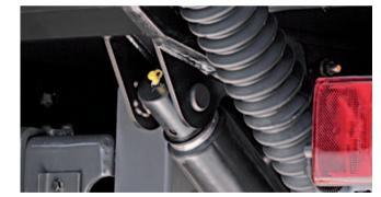
Hydraulic cylinder with **protective tube** or **bellow** (standard) as protection from stone chipping and corrosion. Consistently fast, motorised opening by means of double-action tilting cylinders – even in winter.
