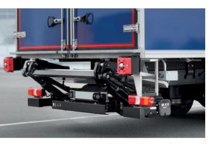
The BC 2000 F is also characterised by a load capacity of 2000 kg and platforms with a height of up to 1510 mm. Like all Falt Cargolifts, the BC 2000 F also remains out of sight below the vehicle while at a ramp and quickly can be ready for use on demand.
