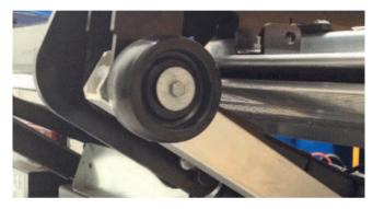
**Ground rollers** (standard) protect the platform from mechanical abrasion with ground contact.
