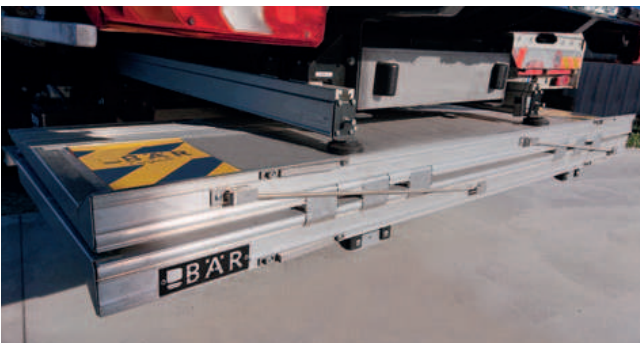
Manual folding of platform tip with spring assistance (standard).
