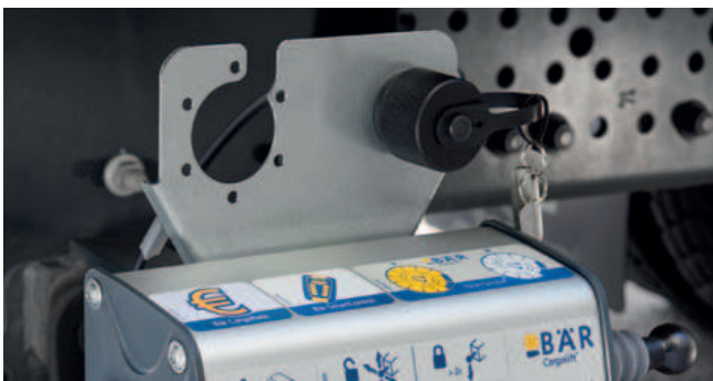
External electrical key switch (option) for mounting on control box holder. Prevents any undesired operation as an alternative to the SwitchKey.
